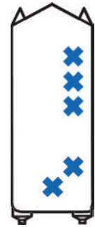
IMPROPER DISTRIBUTION (STARBOARD HEAVY)
